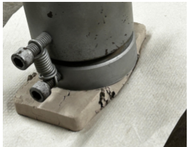
Figure 2: Uniaxial compression test on rectangular lunar bricks, to analyze their mechanical response and failure modes under applied load.
